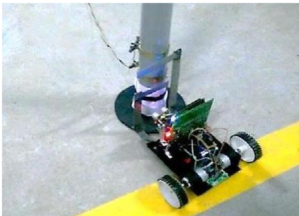
Fig.4(c). Robot docking for recharging
