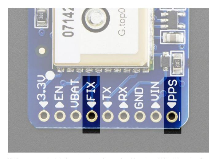
**FIX** is an output pin - it is the same pin as the one that drives the red LED. When there is no fix, the FIX pin is going to pulse up and down once every second. When there is a fix, the pin is low (0V) for most of the time, once every 15 seconds it will pulse high for 200 milliseconds
