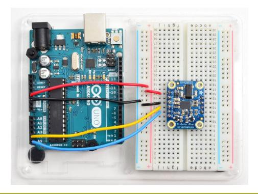
If you're using a Genuino Zero or Arduino Zero with the built in EDBG interface you may need to use I2C address 0x29 since 0x28 is 'taken' by the DBG chip
