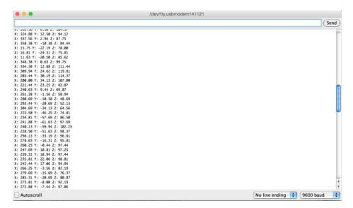
By default, the sketch generates **Euler angle** absolute orientation data, but you can easily modify the data displayed by changing the value provided to **.getVector** below:
